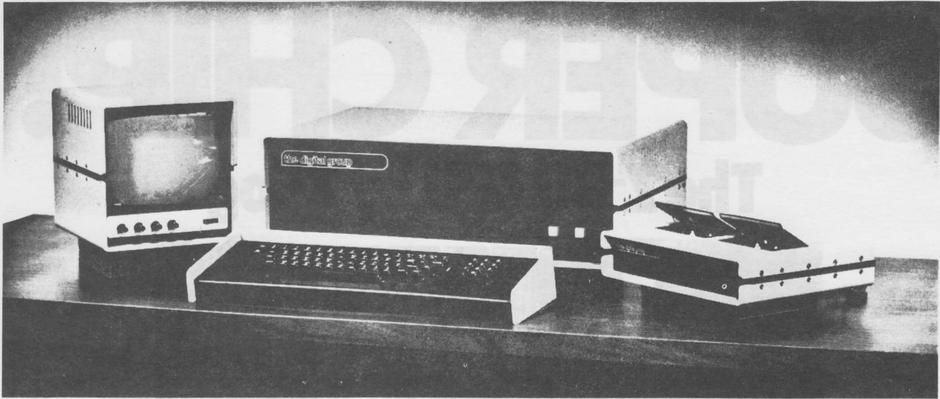
Cabinets clockwise from top: CPU, Dual-cassette drive, Keyboard, 9" Monitor.
