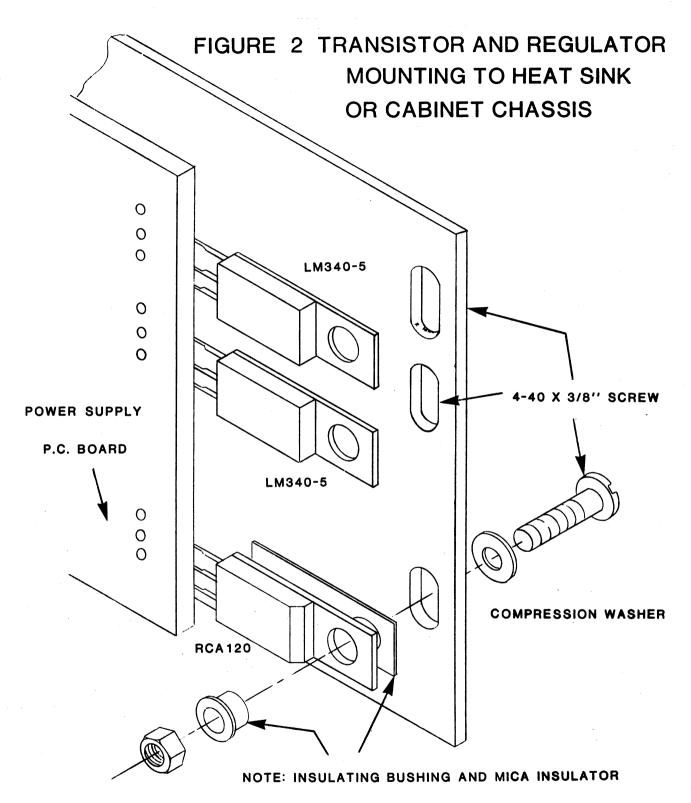
MUST BE USED TO MOUNT Q1-RCA120
